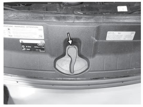
1) Raise the hood. Remove the hood latch release lever by pressing in on the tab on the back side of the lever and lifting the lever up off the hood latch post. Do not close the hood with the hood latch lever disconnected.
