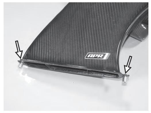
5) Install the spacers on the front side of the APR intake by putting two of the 4mm allen screws through the back side of the holes on the front of the intake and into the spacers. Use a supplied washer on the slotted tab of the intake.
