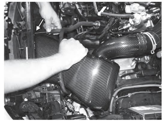
3) Place the APR intake in the car and connect the accordian inlet hose to the back side of the intake. Push down on the intake so the rubber grommet on the bottom of the intake sits on the mounting post underneath. With the intake sitting in its final resting position, mark the back of the radiator core support with an awl or paint pen where the mounting holes for the intake will be.
