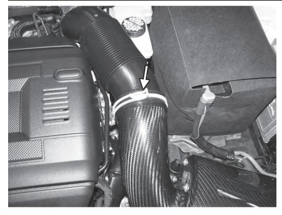
9) Reattach the factory intake tube to the back of the APR intake, and secure with the factory spring clamp.
