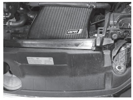
7) Reinstall the upper bumper cover panel by first putting the front side of the panel into the slots on the top of the front bumper cover. Then, lower the cover down into place at the radiator core support. Be sure to replace the hood latch release lever.
