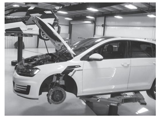
1) Securely lift vehicle. If a vehicle lift is not used, secure the vehicle with jack stands.
