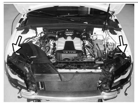
13) Remove 2 T30 Torx screws from top of radiator core support.
