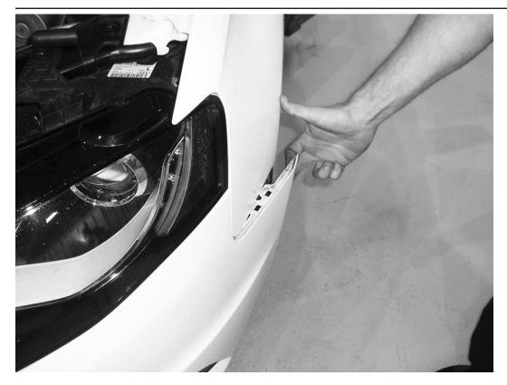
9) Carefully pop the upper corner of bumper cover out. Repeat on opposite side. 10) Carefully pull bumper cover forward and disconnect left and right fog light harness. Remove bumper cover.
