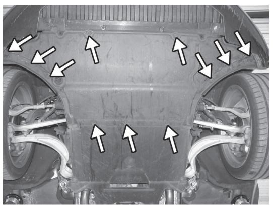
45) Install the 11x quarter turn fasteners onto the belly pan with a screwdriver.
