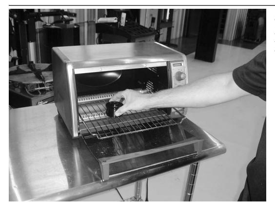
1) Place APR pulley in 350° toaster oven (or equivalent) for one hour (or more). Place the oven on a cart to ensure it can be moved close to the vehicle. Exceeding 350° can damage the finish on the pulley. 2) Securely lift vehicle. If a vehicle lift is not used, secure the vehicle with jack stands. Remove both front wheels.
