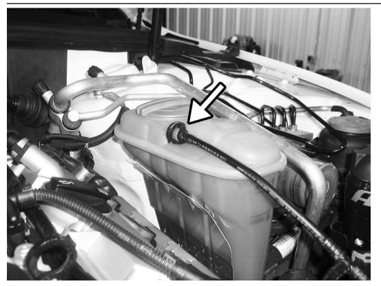
33) Reconnect coolant bleed line to expansion tank.
