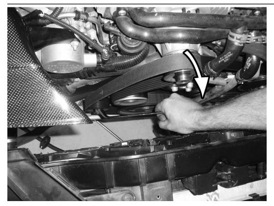
19) Using a 16mm wrench, release tension on supercharger's belt tensioner by pushing down and carefully remove the belt. 20) Remove plastic cap from stock supercharger pulley.
