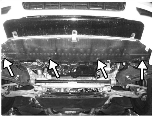
43) Reinstall 4 T30 screws from bottom of bumper cover.
