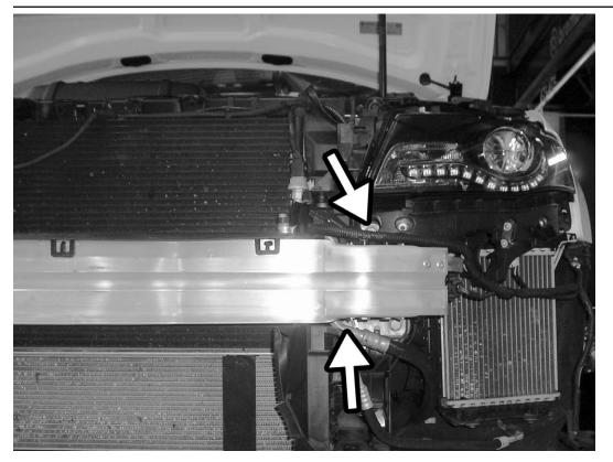
15) Remove the remaining four 16mm bolts holding the core support to the frame rails. 16) Disconnect coolant bleed line from expansion tank.
