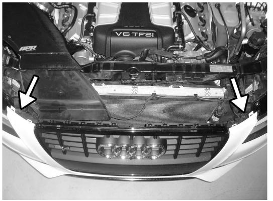
39) Reinstall 2 T25 Torx screws from top of bumper cover.
