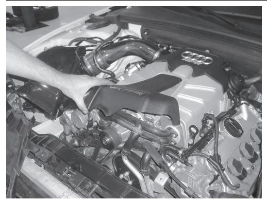
31) Reinstall the engine cover on the front of the supercharger.
