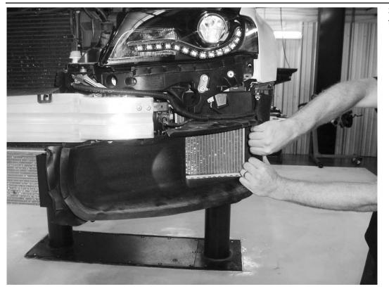
37) Reinstall the radiator ducting on the side radiator.
