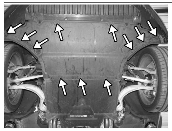
3) Remove the 11 quarter turn fasteners from belly pan with a screwdriver and remove the belly pan.
