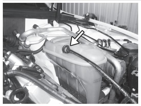
33) Reconnect the coolant hose to the front of the coolant reservoir.
