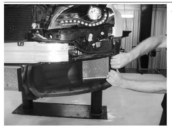
11) Carefully remove the radiator ducting.
