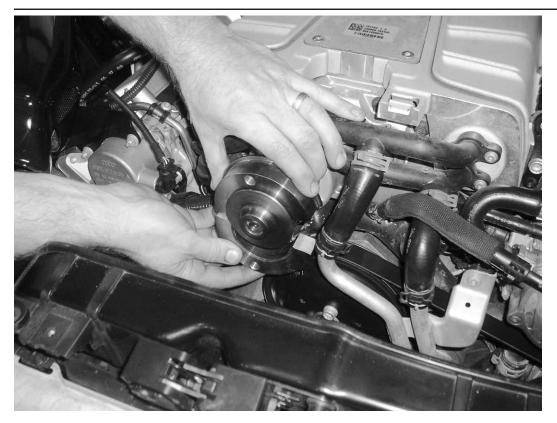
21) Install the supplied "half-moon" pieces around stock pulley. One half moon set fits the stock pulley and the other set fits the APR pulley.
