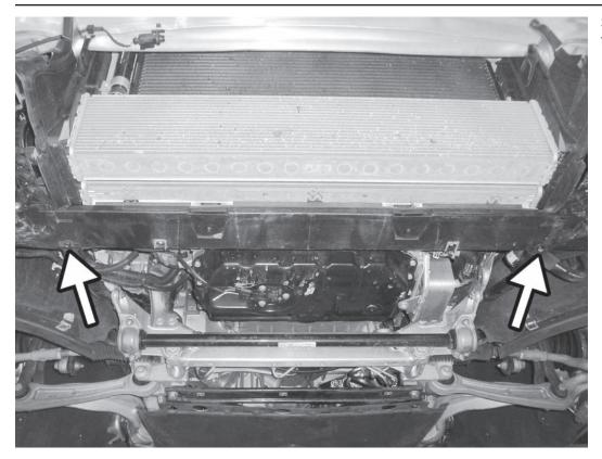
37) Install the 2x T30 Torx screws from bottom of radiator core support.
