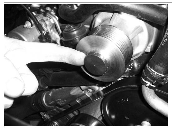
31) Reinstall plastic cap on the APR pulley (if so desired).
