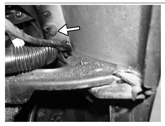
41) Pull back fender liners and reinstall the 10mm bolts on both sides of the bumper cover. 42) Reinstall 2 T25 Torx screws from fender well liner and reinstall the plastic clip.
