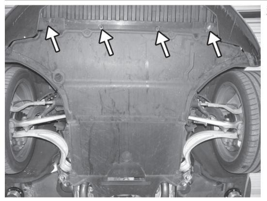
3) Remove the 4x T30 Torx screws from bottom of bumper cover.
