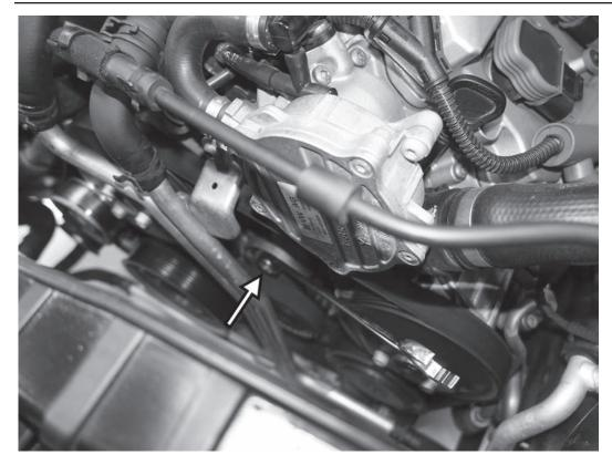
19) Using a 17mm wrench, loosen the tension on the accessories belt by pushing down on the wrench. With tension removed, slip the belt off the alternator pulley on the right side of the engine.
