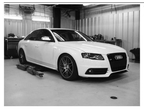
45) Reinstall both front wheels. Remove vehicle from lift (or jack stands). Torque the wheel bolts to 120NM (90Ib-ft). Enjoy!
