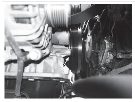
25) Observe how this post on the front of the engine block, just to the right side of the crank pulley, is in the path of the supercharger belt by a few millimeters.
