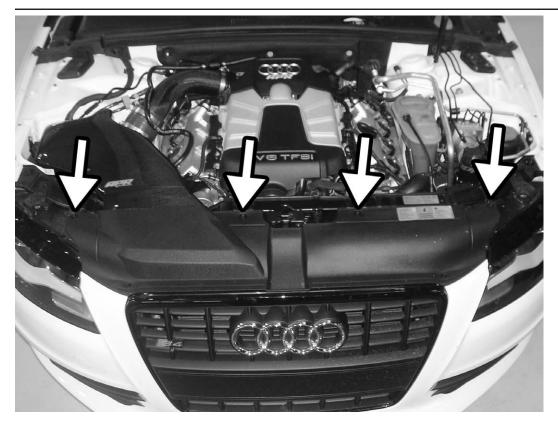
7) Remove 4 T30 Torx screws from upper bumper trim cover and remove the cover.
