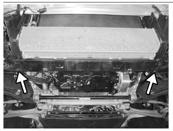
35) Reinstall 2 T30 Torx screws in the bottom of radiator core support.
