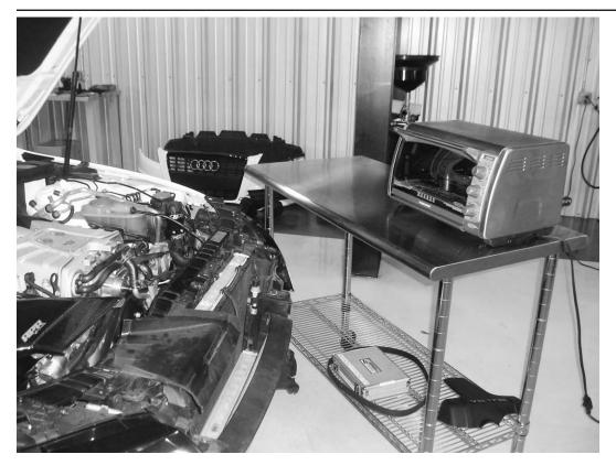
27) Now that the stock pulley is removed, move the oven close to car so that pulley can be installed as quickly as possible.
