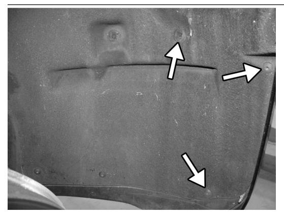
5) Remove 2 outer T25 Torx screws from fender well liner and the outer plastic clip. Repeat on both sides. 6) Pull back fender liner and remove the 10mm bolt from bumper cover. Repeat on both sides.
