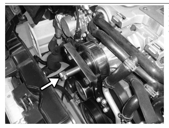
25) Apply a generous amount of Liqui Moly to supplied "screw" on both the end of it and its threads. Hand thread the screw in the "block" until the end touches the supercharger's drive shaft. 26) Install a 1/2" breaker bar into "block" and connect to "screw" with a 1/2" ratchet (19mm). Hold the breaker bar and tighten "screw" until pulley is removed.
