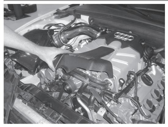
17) Remove front plastic cover from supercharger.
