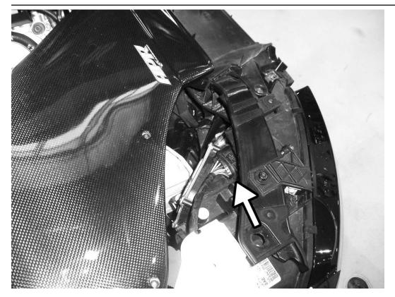
17) Carefully pull the radiator core support forward slightly and disconnect right and left headlight harnesses. The core support can then be pulled fully forward on the two bolts previously installed. 18) Remove front plastic cover from supercharger.
