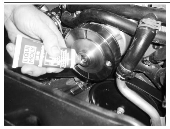
23) Generously apply supplied Liqui Moly to end of the supercharger's drive shaft. 24) Install supplied "block" with the two supplied M10x1.5-50 bolts to "half moon" pieces. Thread bolts hand tight until the "block" bottoms out against pulley.
