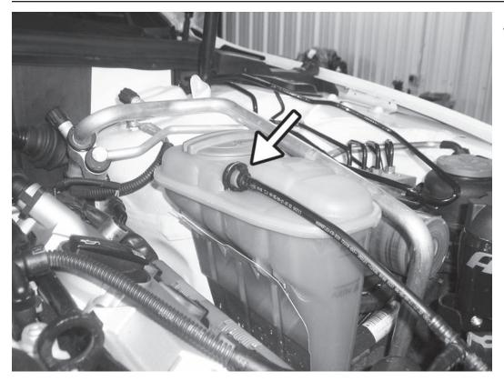
15) Disconnect coolant bleed line from expansion tank.
