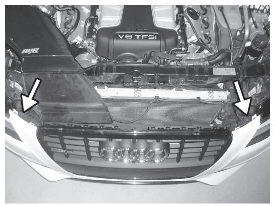
7) Remove 2x T25 Torx screws from top of bumper cover.
