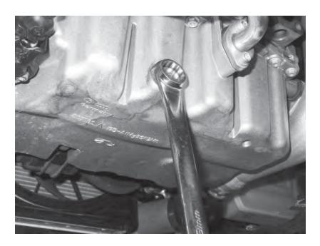
49) Drain the engine oil by removing the 18mm drain bolt from the bottom of the oil pan. It is advisable to change the oil filter on the car at this time as well.
