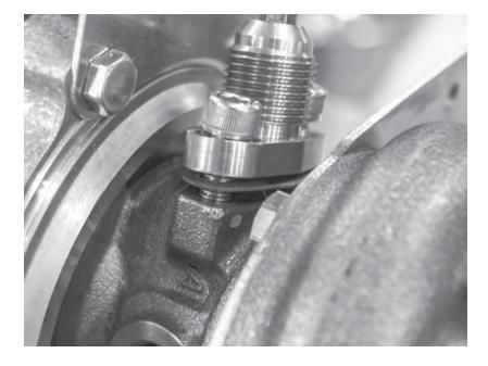
86) Install the fitting on the oil drain line by first installing the gasket, then connecting the fitting with the two 6mm allen bolts and lock washers.
