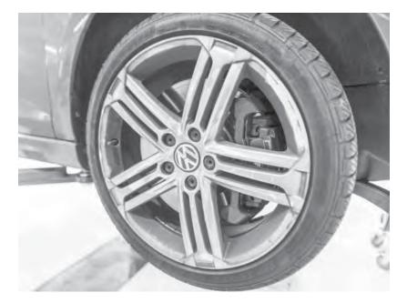
50) Remove the front passenger wheel and set aside.
