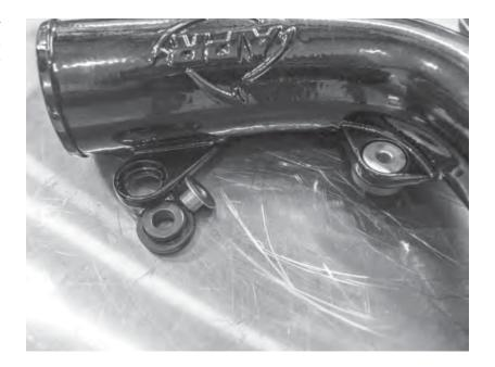
120) Loosely install the APR outlet pipe into the compressor outlet hose and to the passenger side intercooler hose. Secure the APR outlet pipe to the oil pan using the two stock T30 bolts. After confirming the hoses are not kinked, tighten the hose clamps on both ends of the APR outlet pipe and at the intercooler.
