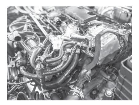
32) Reinstall the three T30 bolts that connect the fuel pump to the cam housing. Tighten these bolts to 89in-lbs in the following sequence: bottom right, top left, top right. Then reinstall the fuel pressure bleed fitting. Reconnect the electrical connector on the top of the fuel pump.
