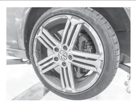
129) Reinstall the front right wheel and torque the lug bolts to 89lb-ft.
