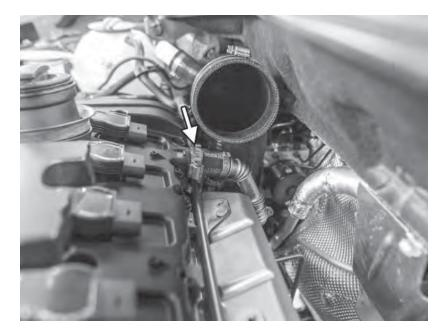
114) Install the breather tube in the APR compressor inlet hose, and connect to the large port on the back of the valve cover. Secure with the supplied clamps.
