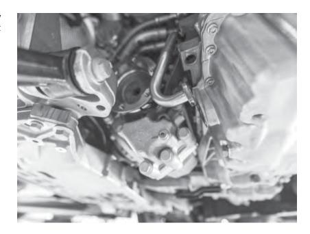
68) Remove the four 15mm nuts that hold the downpipe to the stock turbocharger.
