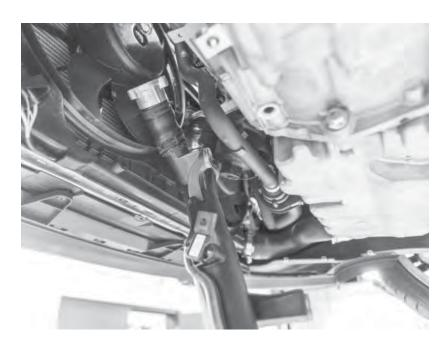
13) Remove the T30 bolt from the bottom of the intake charge pipe and disconnect the lower intercooler hose. Pull the front charge pipe out from underneath the car.
