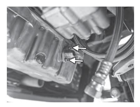
117) Install the oil drain line fitting onto the oil pan with the supplied gasket, 5mm allen bolts, and lockwashers. Install the oil drain line and tighten with a 1" wrench.
