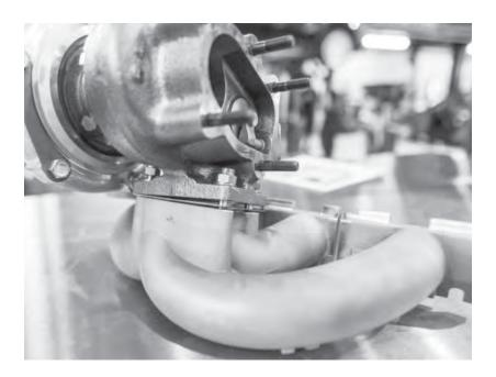
85) Install the gasket on the studs of the manifold and mount the turbocharger with the turbo support bracket facing the inlet ports of the exhaust manifold. Install the four flat washers and then start the locking nuts. Evenly tighten the four 13mm nuts, going in a crossing pattern.
