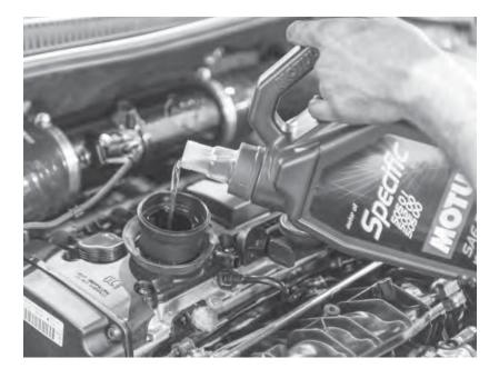
130) Fill the engine with the correct oil and check the level.
