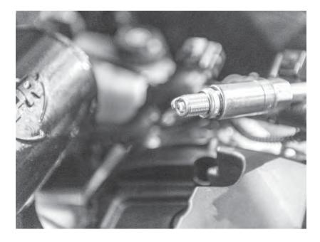
126) Remove the stock coilpacks and sparkplugs. Check the gap on the APR plugs and verify/regap to .028". Install the new spark plugs and torque to 18lb-ft. Reconnect the coilpack wiring harness
