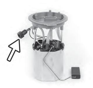
137) Disconnect the bundy fitting from the line that runs from the right side of the fuel tank and connect to the new pump. Being careful not to roll the fuel tank seal, reinstall the locking ring, fuel pump cover, and rear seat in the car.
