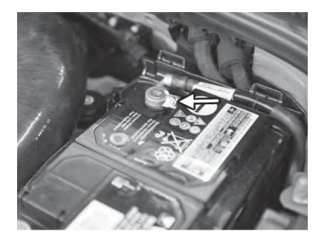
138) Reconnect the negative battery terminal. Let the car sit for at least three minutes with the igniton on and the engine off. This is also a good time to connect to the car with a diagnostic tool to clear any error codes on the car.
