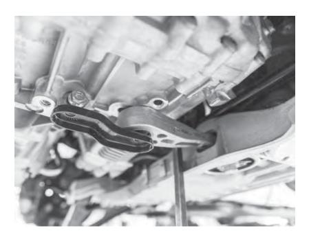
65) Using a pry bar, rock the lower half of the engine forward in the engine bay and use the dogbone mount to keep it forward.
