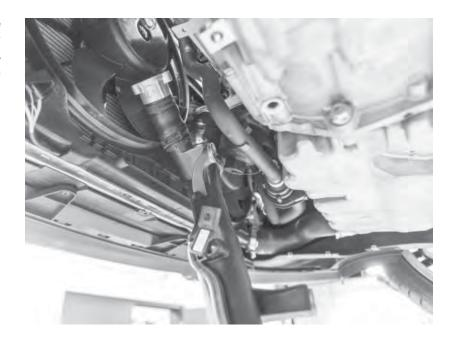
44) Reconnect the lower intercooler hose to the intake charge pipe and tighten the hose clamp. Also tighten both hose clamps to the rubber boot off of the throttle body.
