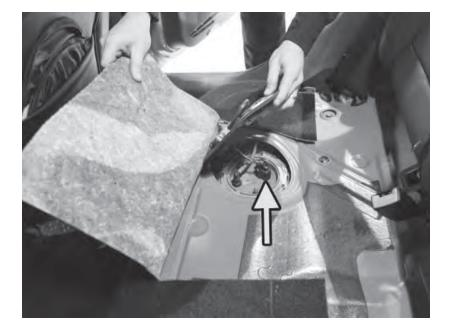
134) Lift the carpet up from the right side of the rear seat tray. Carefully lift the fuel pump cover disconnect the electrical connector to the fuel pump.
