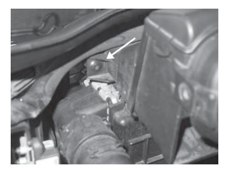
2) Remove the two T25 screws that connect the intake ducting to the radiator support. Then remove the hose clamp next to the round accordion tube, and remove the intake from the car.
