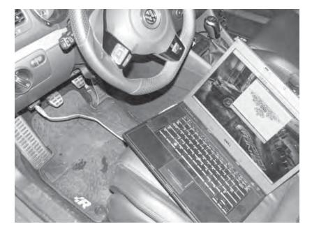
6) It is best at this time to go ahead and program the ECU in the car. If you are an APR dealer, log on to the DirectPort Programming webpage and program the ECU. If the ECU needs to be removed to be sent to APR for programming, do so at this time.
