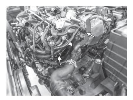
25) On the right side of the intake manifold, disconnect the wiring harness clip from the fuel line. Also disconnect the electrical connectors to the variable intake runner control and the EVAP Purge Valve (N80). Finally, remove both of the upper and lower plastic lines from the vacuum pump.
