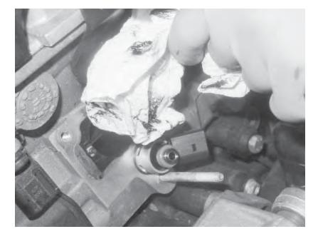
30) Remove the paper or cloth from the intake ports on the block, being careful not to pull the flow separators out of the block.
