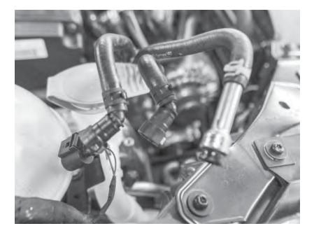
18) The two plastic fittings are disconnected by pushing in on the side of the fitting and lifting the connector off from its mounting location. The metal fitting is removed by lifting the plastic up into the metal housing, and then lifting the line off. The metal fitting is a fuel line, so be sure to use a rag to keep from splashing fuel everywhere.
