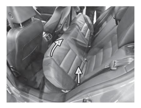
133) Remove the rear seat from the vehicle by lifting firmly up on the front of the seat. Once the front of the seat is raised up and tilted back, Push the seat towards the back of the car, and then you can lift the seat up and out of the car.
