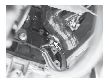
116) Route the coolant return line from the outside of the turbocharger behind the axle heat shield, and loop it around to the correct mounting point on the engine block. Making sure there are crush washers on either side of the fitting of the supplied 16mm banjo bolt, tighten the bolt.
