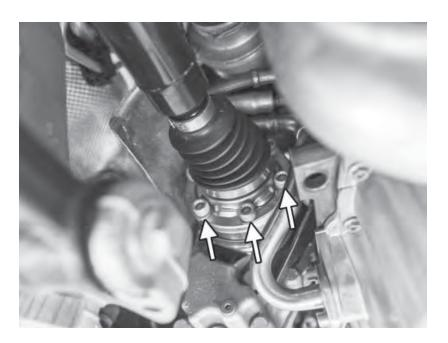
57) Using a 10mm triple square, remove the six inner axle bolts from the passenger side axle. Keep the axle bolts and bolt straps together. Remove the axle from the car.
