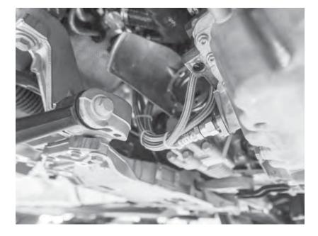
118) Connect all three braided lines (oil feed, oil drain, and coolant return) together with cable ties so they are not hanging loosely.
