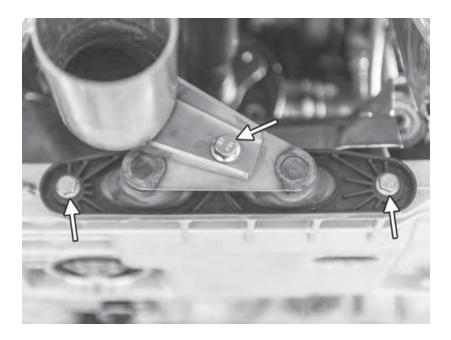
122) Connect the downpipe to the stock exhaust hanger with the supplied bracket. The 15mm bolt connects the bracket to the downpipe, and the two stock 13mm bolts connect the exhaust bracket to the subframe.
