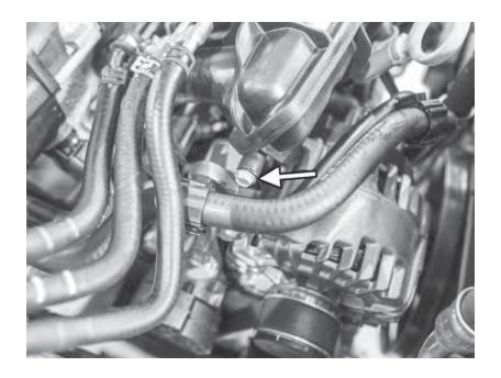
20) Disconnect the 10mm nut from the engine oil dipstick bracket. Then remove the stud the nut was on using a 4mm socket.
