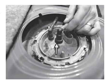
136) Using a large screwdriver and hammer, carefully tap the fuel pump retaining ring counter-clockwise to release the ring. Slightly lift the original fuel pump out of the tank.
