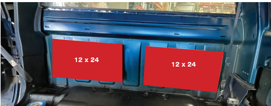
FIG. 3 Rear Bulkhead Install damping material in these approximate locations. The perfect placement is not critical. But good adhesion is key. Make sure to press material in place with roller or other form of pressure to ensure good adhesion. (View from driver side door)
