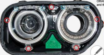
J) Re-install the five 10MM bolts. The locations of the bolts are marked in red circles.
