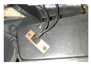
Locate behind original control head the resistor connector, on heater box.
