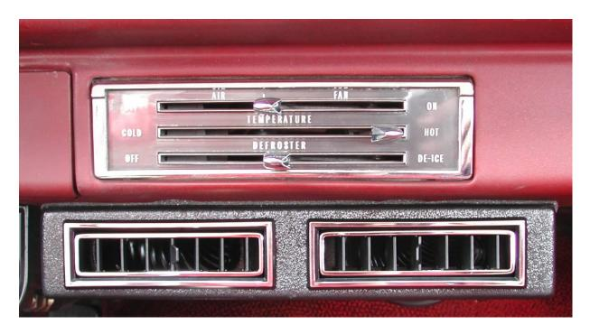
THE PICTURE YOU SEE ABOVE SHOWS THE CONTROLS IN THE DEFROST MODE. THIS MEANS THAT THE AIR WILL BE DISTRIBUTED THROUGH THE DEFROST OUTLETS. THIS ALSO HAS THE TEMPERATURE LEVER IN THE HOT POSITION. WITH THE CONTROLS IN THIS POSITION YOU WILL GET THE AIR THROUGH THE DEFROST OUTLETS WITH THE COMPRESSOR ON.
