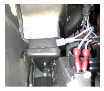
Be sure that defrost outlet from the new unit inserts into the original defrost diffuser.
