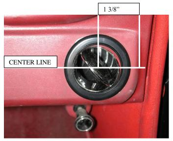
Locate and Drill (1) 2 1/4" dia. hole on passenger lower part of the instrument panel.
