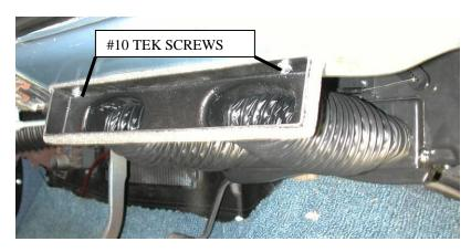
Attach 7 ½" flex hose between center hose adapter and the distribution duct adaptors.
