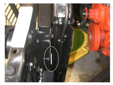
The (4) condenser mounting brackets are clamped between the radiator and its mating bulkhead.
