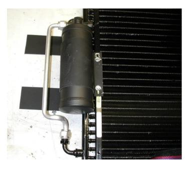
Locate Filter / Drier, Drier Mounting Bracket, Aluminum Liquid tube, (2) #6 orings, and (2) #10 x 3/8" hex head screws.
