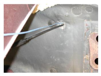
Drill hole for the temperature cable and clutch wire just to right of the firewall pad attachment plug.
