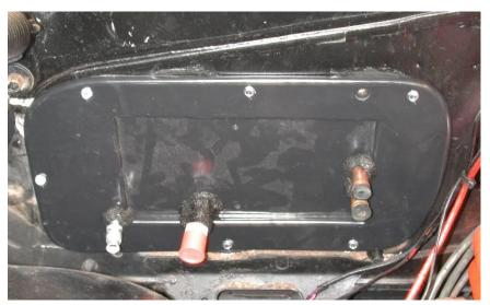
Locate the Firewall Block Off plate, and (6) #10 x 3/4" hex head tek screws.
