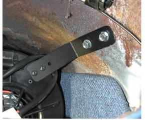
Locate in the hardware sack kit (2)  $\#14 \times \frac{3}{4}$ " tek screws.
