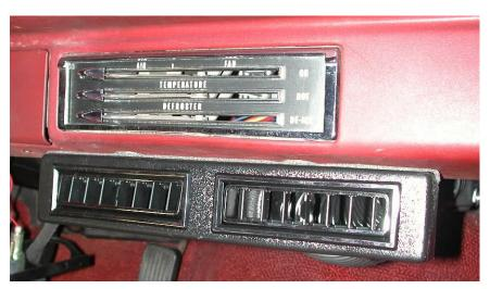
Locate Center Louver Bezel Assembly and (2) #8 x 3/8" pan head screws.
