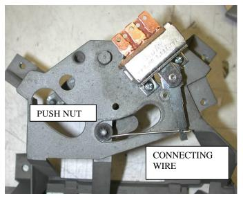
Locate the blower switch, (2) #6 x 3/8" pan head screws, (1) 3/16" push nut and connecting wire from the control sack kit.
