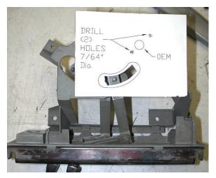
Locate Control Switch Drill Template from the installation instructions.
