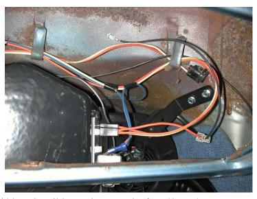
Attach (2) blue wires to the micro-switch and blue pig tail located next to the face / heat door crank arm. Refer to wiring diagram for correct connections.
