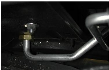
Rotate lower fitting up to the radiator bulkhead. Locate and drill (1) hole 13/16" diameter.
