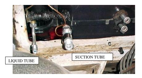
Install the liquid line onto Expansion (TXV) valve as shown. Use #6 o-ring and (2) drops of mineral oil on the o-ring and tighten securely.
