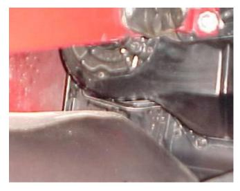
Remove (7) screws around the perimeter of the Blower Housing. The (2) screws around blower motor can be accessed from below and between the fender well and fender. Remove blower assembly.
