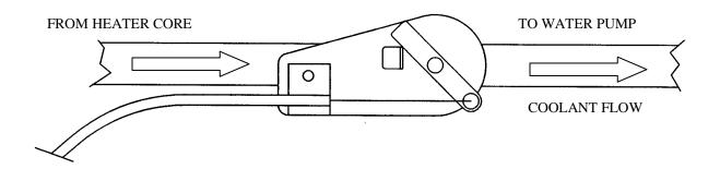
CAUTION: WATER VALVE MUST BE INSTALLED ON HEATER LINE ROUTED TO WATER PUMP.
