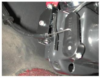
Attach Face / Heat cable to door on side of the center duct assembly using (1) #8 screw.
