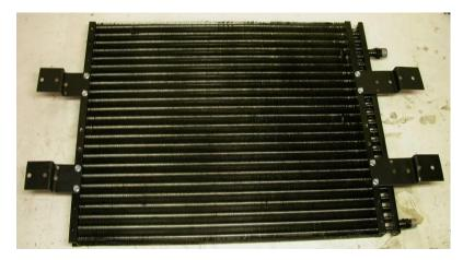
The lower condenser brackets attach to condenser on 3<sup>rd</sup> hole from the bottom.
