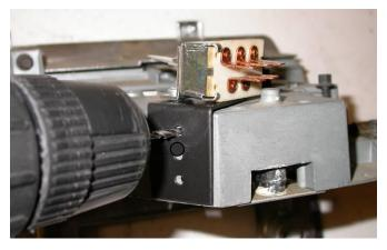
Attach control switch assembly to original control head using (2)  $#8 \times 3/8$ " pan head screws.
