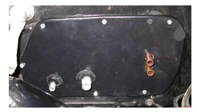
Locate the Firewall Block Off plate, and (6)  $\#10 \times \frac{3}{4}$ " hex head tek screws.
