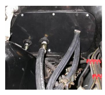
Locate water valve and (3) worm gear clamps from hardware sack kit.
