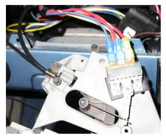
Attach wires to blower switch using the wiring diagram on page 7.
