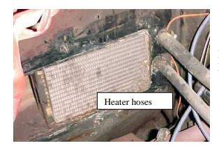
DRAIN COOLANT FROM RADIATOR. Remove Heater hoses from heater coil at firewall.
