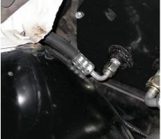
Attach discharge hose to condenser fitting and route to compressor. Attach using (2) #8 o-rings and a few drops of mineral oil.
