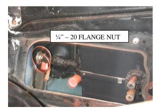
Insert the (1) upper rear Evaporator mounting stud through the original hole as shown. Attach using (1)  $\frac{1}{4}$  - 20 flange nut provided.
