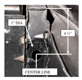
Locate on the center and 4  $\frac{1}{4}$ " down on passenger side of the radiator spacer frame.
