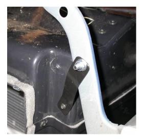
Locate in hardware sack kit the upper evaporator support bracket, (1)  $\frac{1}{4}$  - 20 X 5/8" screw and flange nut.
