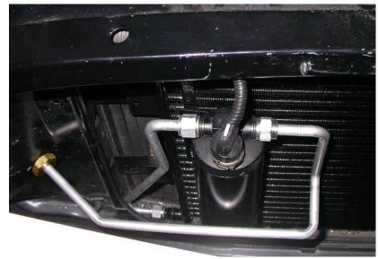
Locate Hi / Low pressure switch assembly, and wire harness. Attach Hi / Low switch assembly using a few drops of mineral oil.
