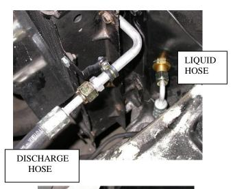
Route Liquid hose Assembly from bulkhead and under battery box. Route inside fender and back to firewall fitting. Attach using (2) o-rings and a few drops of mineral oil.
