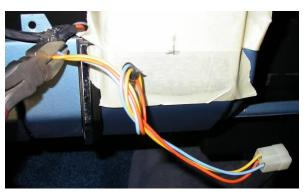
Cut connectors and wires from the original resistor back to main harness.
