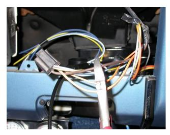
Locate original wire harness that was attached to blower switch. Cut the connector off. Attach (1)  $\frac{1}{4}$ " male spade connector to brown wire.
