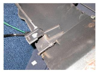
Pull heater box away from firewall and rotate to remove the control cable on back of the box. Discard the original hardware.
