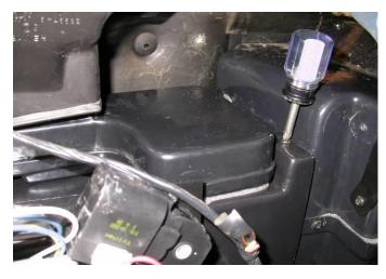
Reinstall passenger fresh air cable to bottom of dash using original hardware. Locate in control sack kit the main wire harness.
