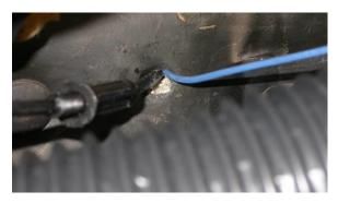
Locate the control head, insert cables through opening in the dash.
