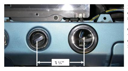
Locate and Drill (1)  $2\frac{1}{4}$  dia. hole on drivers lower part of instrument panel to right of cigarette lighter.
