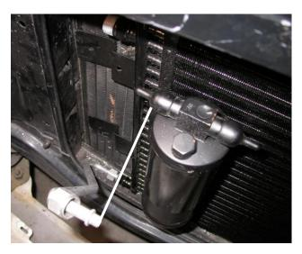
Carefully insert Condenser Assembly through the Radiator Mounting Bulkhead slide assembly to drivers side see picture below.
