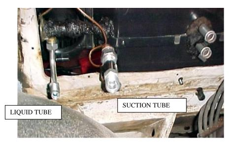
Install liquid line onto Expansion valve (TXV) as shown. Use #6 o-ring and (2) drops of mineral oil on o-ring and tighten securely.
