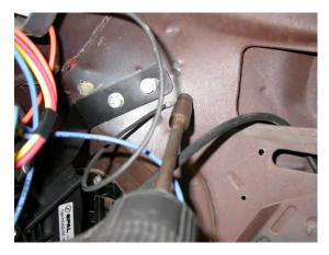
Route wire harness across top of the unit and over to micro switch on the side of distribution duct.
