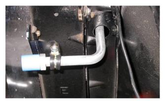
Locate tube support bracket, (1)  $5/16-18 \times \frac{1}{2}$ " hex head bolt, (1) hose clamp, (1) #8 screw and nut.
