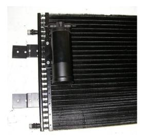
Locate Filter / Drier, Drier Mounting Bracket and  $(2) \#10 \ge 3/8$ " hex head screws.
