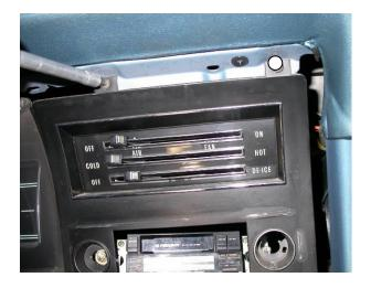
Remove the radio, remove and retain the lower (2) nuts that hold the lower bezel.
