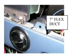
Reinstall fresh air door cable using original hardware.
