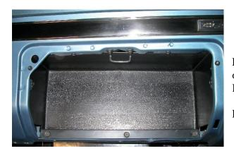
Locate Glove Box provided in the kit and install using original hardware. Install bottom trim using original hardware.
