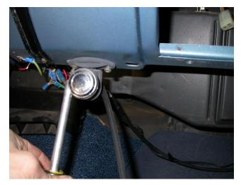
Locate on top of heater assembly accessing through glove box opening the resistor connector.
