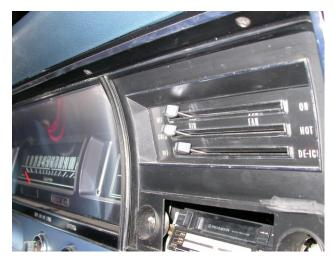
Remove (5) attachment screws across top edge of the instrument trim bezel.
