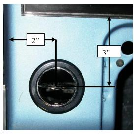
Locate and Drill (1)  $2\frac{1}{4}$ " dia. hole on left side of glove box.
