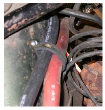
When routing liquid hose attach hose and the return heater hose to shock tower using (1) double clamp and a #10 tek screw.
