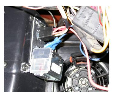
Attach ground wire from blower connector to the body using (1) #10 tek screw.
