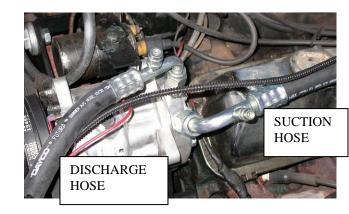
Locate #8 discharge hose and (2) #8 o-ring. Attach end of the hose with 45 deg fitting to the condenser fitting and end with the service port to compressor.
