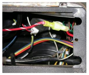
Locate orange wire with bullet connector that was attached to the original blower motor. Cut off the connector and add a ¼" male spade connector.
