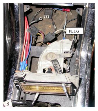
Insert electrical wiring and control cables into the center console.
