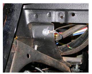
Locate black wire with a ring terminal that is attached to the relay on the duct.
