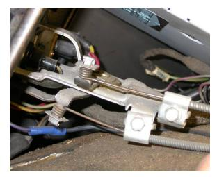
Remove cables from back of the control head. Retain original hardware for the cable clamps.
