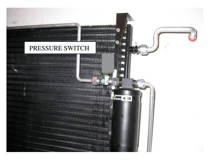
Slide condenser between radiator and the radiator support. Let hange on the upper brackets.
