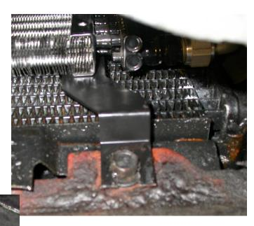
Locate (1) 3/8" tube clamp and (1) #10 x 3/4" tek screw.
