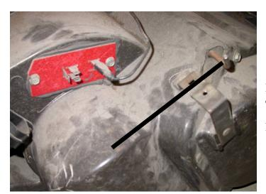
Disconnect electrical plug from resistor on the heater box.
