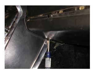
Remove and retain screws along console that holds the lower dash panel.
