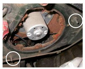
Remove (3) nuts from the heater mounting studs.
