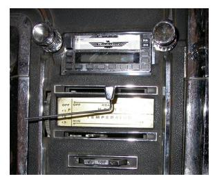
Remove (6) screws that hold the center console cover. NOTE: (2) of the screws are under arm rest.
