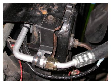
Locate discharge tube support bracket, #8 hose clamp and (1) #10 x 3/8" pan head screw.
