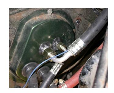
Locate #10 suction hose and (2) #10 o-rings. Attach hose to fitting on the block off and end with the service port to the compressor.
