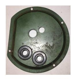
Install service cover inserting heater hoses through the grommets and a/c tubes through the holes.
