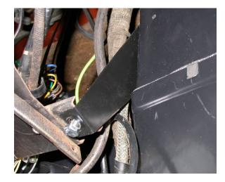
Loosely install original bolt into the front brace. This will hold unit in place while you attach the blower support brace.
