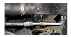
When routing suction hose tywrap hose to the body brace beside the air cleaner.
