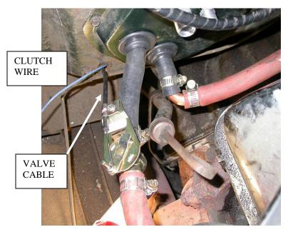
Route longest of the control cables across back of the evaporator and out through original heater mounting hole. Attach to the water valve.
