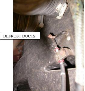
Remove control cable from center of heater box next to the defrost ducts. Discard the cable.
