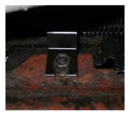
Locate left bottom condenser mounting bracket and slide into the bottom radiator mounting bolt.
