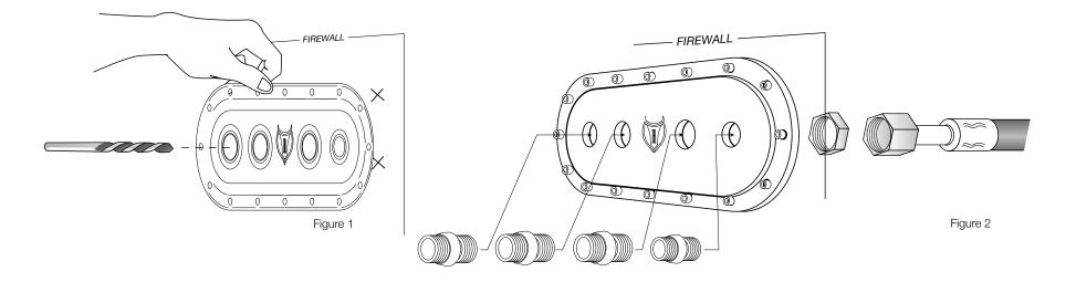
Step 1: Determine a mounting location for the billet plate on your vehicle (see figure 1). Using the plate (or the included template) carefully mark and drill a 5/8" diameter hole for the liquid hose fitting, and 7/8" holes for the heater and the suction hose fittings.
