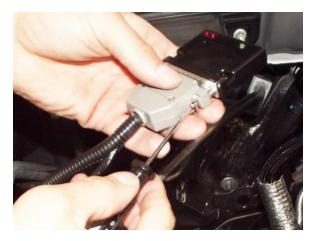
**Important:** Disconnect the negative terminal of the battery before installing this product. If you do not disconnect the battery the factory computer will not learn the correct starting pedal position.
