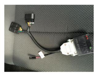
**Connect the Assembly:** Attach the black PedalMAX device to the wiring harness. Apply the supplied dialectric grease on the connector pins and plug the device into the 25-pin connector and secure it with the two small screws. Use the supplied screwdriver.
