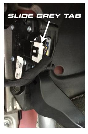
**Step 3:** Plug the PedalMAX device in-line between the pedal position sensor and OE wiring harness by connecting the male and female PedalMAX connectors to the Original Factory connector and sensor.
