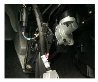
**Step 4:** Secure the PedalMAX unit using the (2) supplied cable ties. The device should not be hanging loosely or unsecured. Do not attach or mount to any moving assemblies such as the steering column. Do not attach or mount to the air conditioning return line shown in the image, this line is extremely hot under operating conditions!
