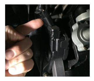
**Step 3:** Plug the PedalMAX device in-line between the pedal position sensor and OE wiring harness by connecting the male and female PedalMAX connectors to the Original Factory connector and sensor.
