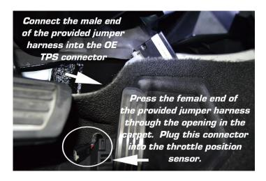
**Step 6:** Tuck the JMS module into the pocket located directly behind the opening in the carpet, then press the carpet back into place. Note: If this is done correctly, the carpeting will look completely OE.
