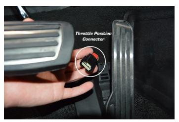
**Step 3:** Pull the carpet from behind the pedals back, the carpet is only set in place and should NOT take any force to pull back.
