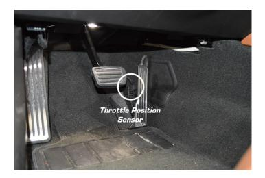
**STEP 2:** Unplug the wiring harness from the pedal position sensor.
