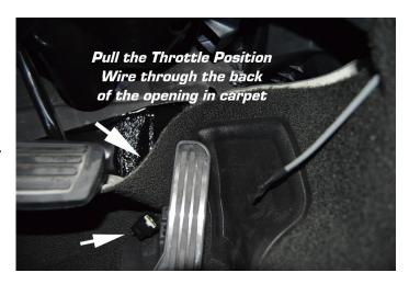
**Step 5:** Connect the Male end of the supplied Jumper Harness to the Female TPS connector (the connector that was just pulled through the carpet). Then push the Female end of the provided jumper harness through the opening in the carpet and connect it to the Throttle Position Sensor.
