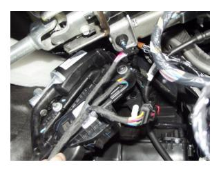
**Step 4:** Secure the PedalMAX unit using the (2) supplied cable ties. The device should not be hanging loosely or unsecured. Do not attach or mount to any moving assemblies such as the steering column.
