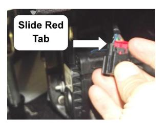
**Step 3:** Plug the PedalMAX device in-line between the pedal position sensor and OE wiring harness by connecting the male and female PedalMAX connectors to the Original Factory connector and sensor.
