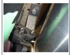
5. Secure the hitch to the lower bumper support using a M8 hex bolt, 5/16" lock washer and 5/16" flat washer into the existing weld nut on both sides as shown. Insert the 7/16" hex bolts with 3/8" flat washers into the existing holes as shown and secure with 7/16 hex flange nuts.°
