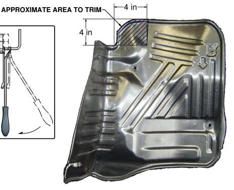
**HEAT SHIELD TRIM DIAGRAM** (BOTH SIDES)
