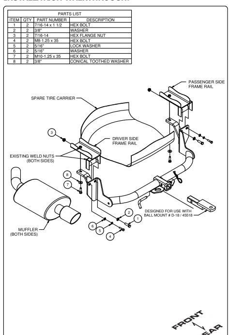
Lower the exhaust by removing the (3) rear most rubber isolators on each side of the exhaust. Gently spread the exhaust to allow the mufflers to pass by the spare tire carrier. Support the exhaust system to prevent damage. (See Rubber Isolator Removal Diagram.)
