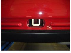
12. Align bumper cover and pull back on the fender flairs. Re-attach wiring harness to bumper cover. **Note:** Side markers need to be re-attached to the wire harness prior to securing bumper cover. Reinstall all (11) fasteners removed previously and snap fender flairs back into place.
