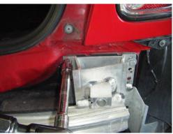
8. Remove the (2) plastic nuts securing the divider panel to the aluminum bumper beam. Return the plastic nuts, divider panel, and hard foam energy absorber to owner.
