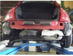
9. Raise the hitch into position by aligning the holes with the weldnuts. <u>Note</u>: The hitch will fit firmly between the spare tire and the rear panel.
