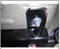
6. Torque all M10 bolts to 48 lb-ft and all 1/2" fasteners to 110 lb-ft.
