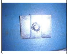
5. Raise hitch into position onto carriage bolts installed in step 4 being careful not to push the bolts back into the trunk. Loosely install the (2) 1/2" hex flange nuts and the (2) M10 hex bolts with (2) conical tooth washers shown on sheet 2.
