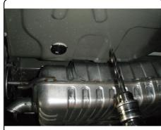
4. Using silicone caulk, place a 1/4" bead around the holes in the trunk pan, on the (2) CM-SP34, (1) CM-SP28, and (1) CM-SP50 spacers. Place the spacers in the trunk directly center over the trunk pan holes. Place the (2) 1/2" carriage bolts into the spacers.
