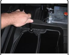
2. Remove the underbody panel by removing (8) 7mm hex head screws, (2) T-15 button head Torx screws, and (1) plastic body panel fastener.
