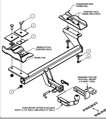
1. Clear contents from trunk and remove the plastic trunk pan insert by removing (4) 10mm nuts.
