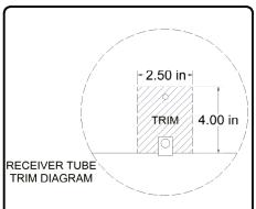
8. Notch the front of the underbody panel (side plate trim diagram shown below) for side plate clearance.
