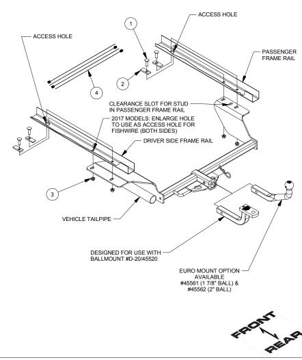
1. Fishwire CM-SP2 spacers and 7/16-14 carriage bolts through access hole in frame rail and down through attachment hole, (2) places, each side.
