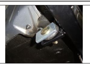
6. Torque 7/16" hardware to 70 lb-ft. Torque 1/2" hardware to 110 lb-ft.
