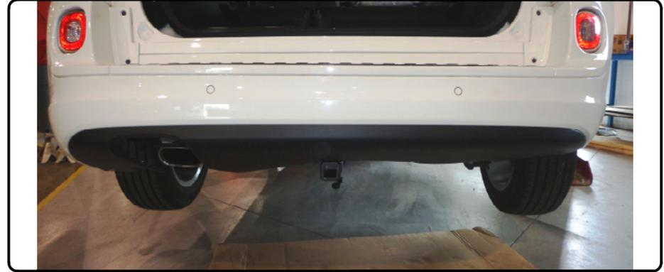
8. Trim approximately 5" x 2 1/2" area at the center of the fascia as shown in the trim diagram. Reassemble the rear fascia by following Steps 1-2 in reverse.
