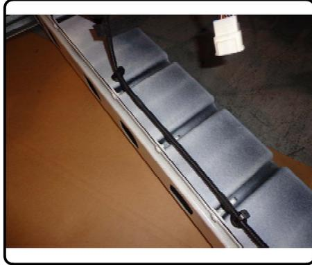
4. Drill out outboard passenger side rivet with 13/64" bit and trim 2 1/2" x 6" plastic area with shears or a rotary tool as shown. This will allow passenger side plate to sit flush when mounted.
