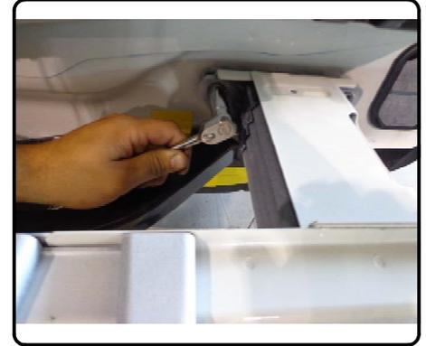
6. Fishwire 1/2" carriage bolts and spacers through bumper access holes and out center support brackets. Tighten 1/2" nuts to secure center support. Locate front mounting plate to secure electrical housing bracket and secure with T30 torx bit that was removed from vehicle in Step. 1.
