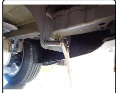
2. Raise hitch into positon and secure the hitch front hole to the weld stud with nut removed in Step (1).
