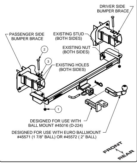
1. Remove existing 8mm nut from the inner most weld stud on frame flange, both sides.
