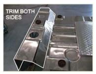
HEAT SHIELD TRIMMING
