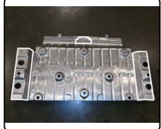
6. Raise hitch up to frame rails and align forward mounting hole with large frame access hole. Mark and drill rear frame mounting hole (17/32") on both sides using the hitch side plates as a template.
