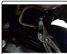
4. Remove (2) plastic fascia supports using a 10mm socket and unclip from bumper beam.
