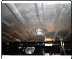
5. Mark heat shield as shown to trim for receiver tube clearance (6" wide) and to allow access to both frame rails. Reattach trimmed heat shield using (8) of the nuts removed in Step 4.
