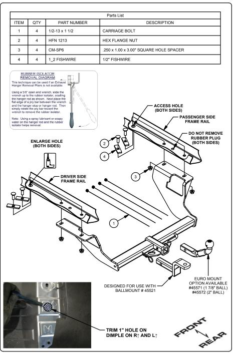
1) Lower exhaust by removing (5) rear rubber isolators. See RUBBER ISOLATOR REMOVAL DIAGRAM. If needed to access outside hangers remove plastic underbody panels by removing plastic fittings (7 per side). NOTE: Support the exhaust as required.
