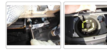
Reinstall the (2) outer screws through the bumper fascia and into the trunk pan.
