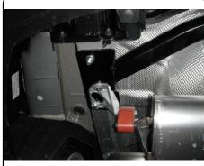
5. Torque all M8 hardware to 23 ft-lbs. Torque all 7/16" hardware to 70 ft-lbs.
