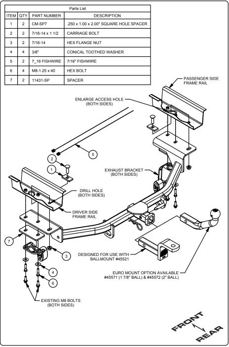
1. Remove (4) bolts and lower the (2) rear exhaust brackets, return bolts to owner.
