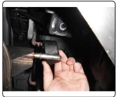
2. Using a 10mm socket, remove plastic fascia tab supports attaching fascia tab to bottom of frame rails on driver and passenger corners of vehicle. Return both supports and (2) support screws to vehicle owner. Retain the remaining (2) support screws for reinstallation.
