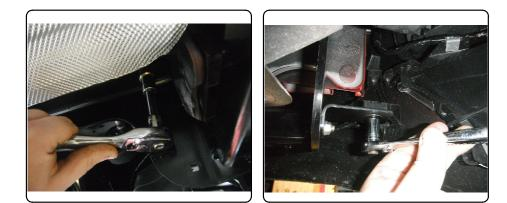
8. Raise exhaust back into position and reattach all exhaust hangers.
