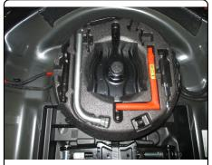
9. Reinstall hands-free trunk sensor into clips. Guide sensor across trim area and behind mounting plate. Reinstall (2) hex nuts removed in STEP 1 with a 10mm socket.
