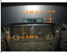
6. Raise hitch into position, guiding bolts through slots in hitch. Loosely secure hitch into position using (4) 1/2" hex flange nuts.
