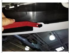
2. Raise hitch into position using (1) 7/16" bolt and (1) CM-SP16 spacer on each side. Loosely secure using (2) 7/16" hex flange nuts.
