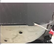
Remove (4) nuts from the bumper beam, (2) on each side, using a 15mm socket. Unpin electrical wire from bumber beam. Set aside hardware for reinstallation.
