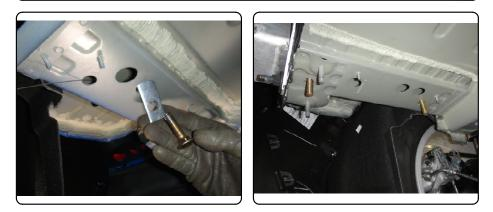
4. Raise hitch into position over exhaust and secure with 7/16" flange nuts. Torque 7/16" bolts to 59 ft-lbs. Reinstall exhaust using nuts removed in Step 1.
