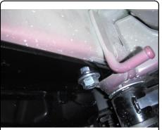
4) Torque all 7/16" fasteners to 70 lb-ft, and all 1/2" fasteners to 110 lb-ft.
