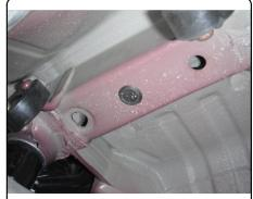
2) Fishwire 7/16" carriage bolts and CM-SP11 spacers into position first and reverse fishwire 1/2" carriage bolts and CM-SP6 spacers into position afterward. (enlarge access hole as necessary)
