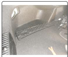
7. Remove (2) plastic fasteners which hold trunk floor cover in position. Remove floor cover.
