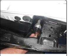
23. Use tape measure, marker and cut wheel to remove a 1.63" wide x 1.25" deep rectangle from center bottom portion of fascia panel.
