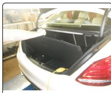
8. Pull away the trunk liner to gain access to the taillight mounting area.
