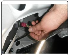
11. Carefully pull taillight rearward and remove, repeat on other side. Use a trim panel tool to ease the process.
