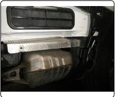
14. Remove (2) screws from rear exhaust hanger using a 3/8" 12 point socket or E12 external torx socket and rotate hanger down. Repeat on other side.
