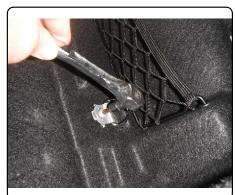
6. Remove (1) panel per side which covers the taillight wiring and lower cargo nets.
