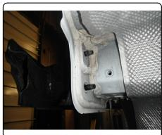
16. Remove (4) inner bumper beam hex flange nuts using a 16mm socket. These are located inside the trunk under the floor liner. Remove bumper beam.
