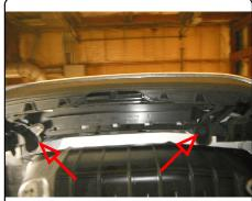
2. Remove (5) plastic push rivets from each rear wheel well. To remove pry the center pin outward, then pry out the rivet. NOTE: (1) rivet per side is under the wheel well liner.
