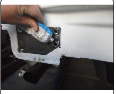
19. Raise hitch and bumper beam into position and attach to outer (4) bumper beam studs using the existing M10 flange nuts.
