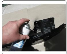
18. Apply silicon on outside of vehicle around (4) inner mounting holes. NOTE: This is important to prevent exhaust fumes from entering the vehicle.
