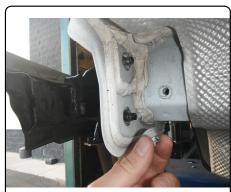
20. Insert (4) supplied M10 hex bolts with (4) M10 washers through bumper beam, hitch and vehicle.
