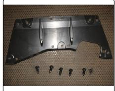
2. Remove (2) remaining underbody panels by removing (8) plunger fasteners, starting near the outside of the vehicle. Remove (2) plunger style fasteners that secure the fascia tabs to the trunk pan. Save panels and fasteners for reinstallation.
