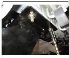
6. Raise exhaust back into position and reinstall the (4) rubber isolators.
