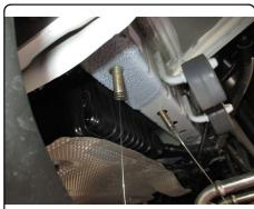
4. Carefully, raise the hitch into position over the exhaust and onto the carriage bolts. Loosely install the supplied hex flange nuts. Push the hitch as far rearward on the vehicle as possible to give as much clearance as possible to the muffler and exhaust components.
