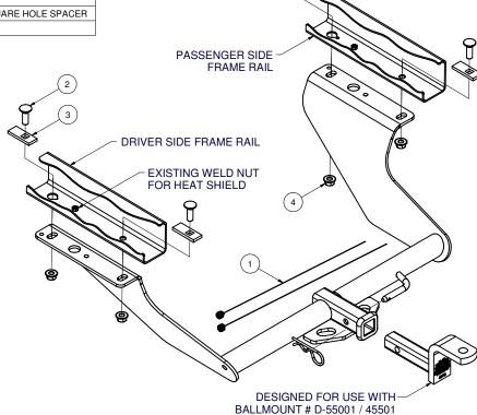
REMOVE PLUG AND MODIFY USING DIE GRINDER (OR ROUND FILE) TO ALLOW INSERTION OF 1/2-13 BOLTS AND CM-SP10 SPACERS INTO FRAME RAIL -
