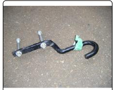
4. Insert 4" hex bolts with washers into the frame rails from the outside. Raise the hitch into position between the frame rails. Push front bolts through mounting plates and loosely install 1/2" flange nuts.
