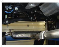
3. Temporarily remove heat shield by removing (4) nuts. (**Note**: If tow loop is present remove and return to vehicle owner.)
