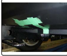
7. Install remaining 1/2" bolts and secure hitch with hex flange nuts. Torque all 1/2" fasteners to 75 ft-lbs.
