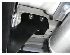
5. Torque all 7/16" fasteners to 70 lb.-ft and all 1/2" fasteners to 110 lb.-ft. Reinstall heat shield and exhaust removed in step 2.
