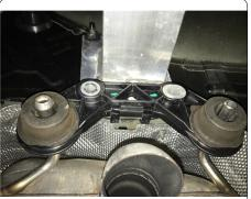
2. Remove heat shield using needle nose pliers to loosen (4) speed nuts on driver side and (2) speed nuts on passenger. Trim heat shield using aviation shears as shown in Heat Shield Trim Diagram.
