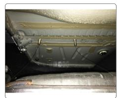
Remove (1) screw on each side using 7mm socket attaching rear fascia to vehicle.
