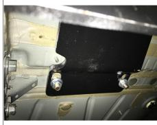
6. Reinstall vehicle exhaust bracket on hitch mounting plate and secure using (2) M10 x 70 and (1) CM-SP1 on each side.
