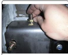
8. Torque all 1/2" fasteners to 110 lb-ft. Torque all M14 fasteners to 126 lb-ft.
