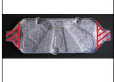
4. Remove the (6) plastic hole covers if present and using a die grinder, enlarge the rearward most holes in the bottom of the frame to allow the supplied carriage bolts and spacers to pass through. Fishwire all (6) 1/2" carriage bolts and CM-SP10 spacers into the mounting positions as shown in the diagram above.
