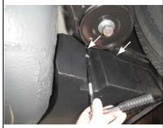
2. Locate (2) weldnuts near the end of each frame rail. Clean weldnuts of debris and rust to ease hitch installation.
