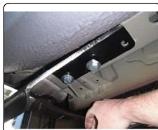
4. On the driver side frame rail fishwire a 7/16-14 x 1 1/2" carriage bolt and CM-SP2 spacer through the access hole and into the existing hole in the bottom of the frame rail. Secure with 7/16" flange nut.
