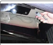
5. Torque all 12mm hardware to 86 ft-lbs. Torque all 7/16" hardware to 70 ft-lbs.
