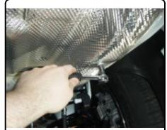
4. Raise hitch into position by raising passenger side of hitch over exhaust and secure into position with supplied M10 bolts and 7/16" conical toothed washers, as shown. NOTE: If the vehicle fascia prevents the hitch from being raised completely into position see trim diagram on page 2.
