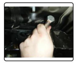
6. Torque 7/16" hardware to 70 lb-ft and M10 hardware to 48 lb-ft. Raise exhaust and spare tire back into position.
