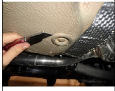
4. Insert the 1/2" carriage bolt and spacer into the trunk pan holes. Apply caulk/sealant to the area between the trunk pan hole and hitch. Raise hitch into position and lightly secure with 1/2" hardware.
