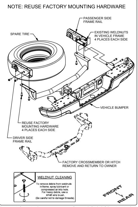
Lower spare tire using the vehicle service tools located in the cab of the truck. Remove the center bracket by removing (4) bolts with a 13mm socket. Return bracket and hardware to customer and raise spare tire back into position.
