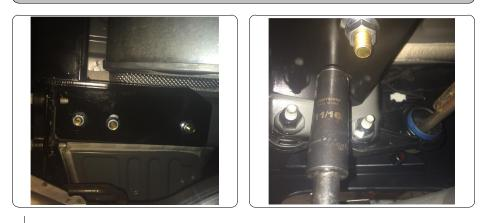
4. When hitch is not in use reinstall access panel removed in Step 1.
