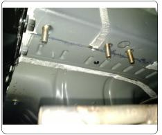
**FISHWIRE TECHNIQUE** NSERT COILED END OF FISHWIRE TOOL THROUGH HITCH MOUNTING HOLE IN VEHICLE FRAME RAI AND OUT THE ACCESS HOLE. PASS COILED END OF FISHWIRE THROUGH SPACER AND THREAD BOLT INTO COIL. KINK WIRE TO KEEP SPACER SEPERATE FROM BOLT AS SHOWN. PULL FISHWIRE, SPACER, AND BOLT THROUGH FRAME AND OUT MOUNTING HOLE. USE FISHWIRE TO GUIDE HITCH DURING MOUNTING AND PREVENT LOSS OF BOLT SPACER INSIDE FRAME RAIL. \*\*NOTE: SOME VEHICLES MAY FISHWIRE THROUGH END OF FRAME\*
