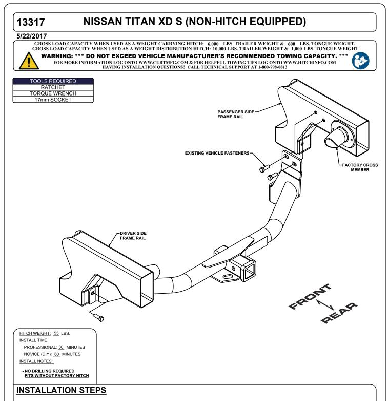
1. Remove (10) M12 bolts from the vehicle using a 17mm socket as shown above. Loosening the (2) remaining bumper bolts and (4) spring shackle reinforcement bracket bolts will aid bolt removal.
