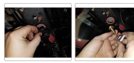
4. Raise hitch into position and feed fishwires through center hole on the hitch. Remove fishwires and loosely secure with 7/16" hex flange nuts.
