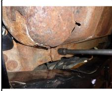
2. Move nut plates into location aligned with holes inside frame rail.
