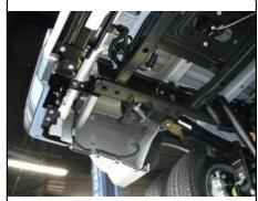
2. Place a carriage bolt and spacer into each bolt location from inside the frame rail as shown.
