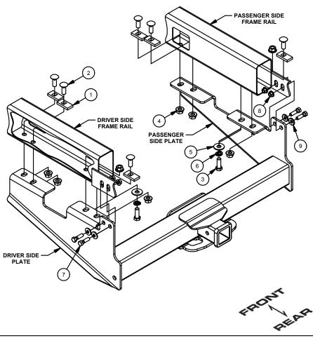
Note: To ease installation, temporary removal of the spare tire is recommended. A 21mm socket will be needed.
