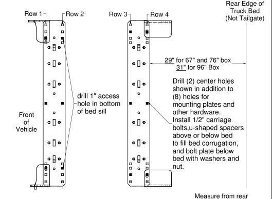
edge of truck bed to rear edge of mounting
